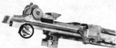
Figure 10. Position of the selector for removing the connector assembly (rifle modified for selective firing).
